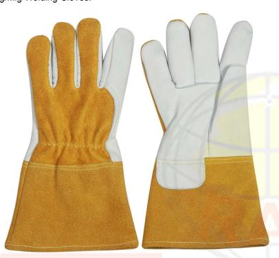
Palm Premium Cowhide Leather back Cowsplit have good strength and abrasion resistant and referred to as strongest leather. Soft and good thick, sewn with Kevlar thread, wing thumb with full lined, and this is great for welding works.
