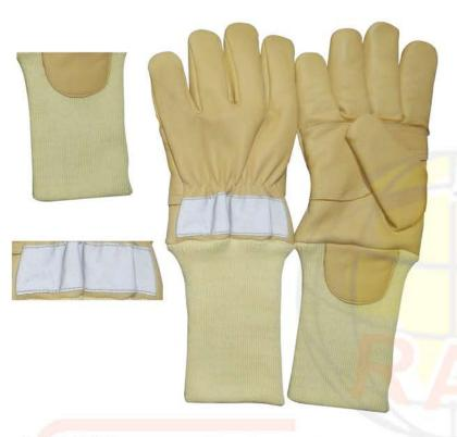
RSAFE-2500C4 Flame retardant (FR) + Water repellant treatment Goatskin leather Gloves, leather reinforcement on palm, Kevlar@ knitted wrist with goatskin leather reinforcement, HI-VIZ refelector tape back of hand, Keystone thumb, DuPont™ Kevlar® lined ANSI A4.
